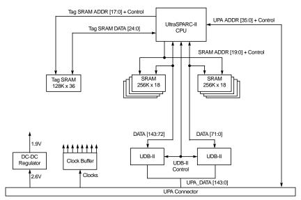
Figure 1. Module Block Diagram
